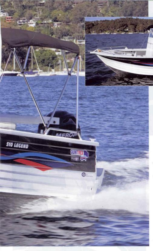
Design: Like all 'offshore' Quintrex models the 510 Legend features the unique fared bow and Millennium hull that deflects spray and makes for a nicer, more level ride. It features a fairly shallow vee hull, however relies on the hollowed bow entry to improve ride in choppy water.
